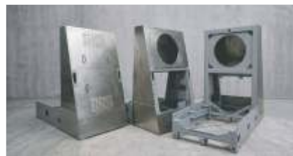
Machined Structure with cladding
